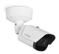
The camera is a versatile and professional surveillance camera for outdoor monitoring. It offers a 1/2.8" sensor and HDR technology at HD 1080p resolution with a built-in intelligent infrared illuminator that provides high performance in dark environments. Built-in Intelligent Video Analytics Pro (IVA Pro) enriches full situational awareness and triggers relevant alerts.
